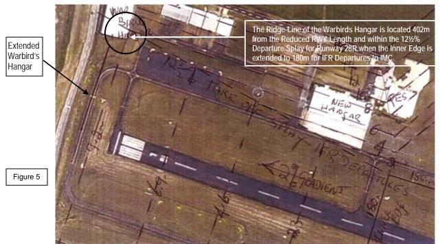
The Warbird's Hangar Roof is within the Take-Off Splay for 28R IFR Departures in IMC & Penetrates the 2% Gradient
