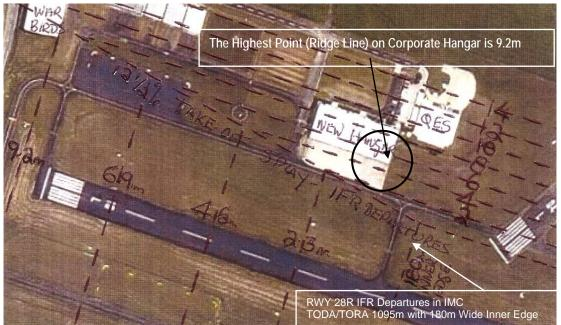
When runway 28R's Inner Edge is 180m for IFR Take-Off in IMC, the Corporate Hangar's highest point penetrates the Transitional Surface by 2.2m. runway 04L's Transitional Surface is shown on Page 9 and indicates the EMQ Building Penetrates runway 04L/22R Transitional Surface by approx.3m.
