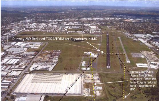
Runway 28R IFR Take-Off Splay together with the adjusted 28R Public Safety Area (PSA) for 28R IFR Departures showing precisely how the Warbirds and the Corporate Hangar breach standards and current PSA\* legislation.
