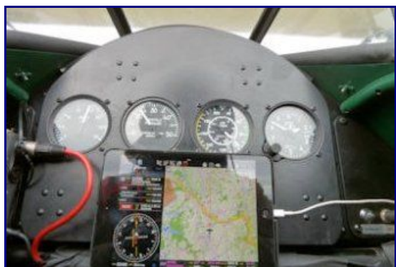
Photo: Cockpit of 1940s era biplane, with modern addition of satellite navigation. (Supplied)
